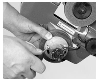
When it is time to replace the wheel follow these instructions. Unscrew the caterpillar screw that is located on the wheel supporter, remove the wheel from the shaft of the motor, then unscrew the three screws that keep the plastic tight.. Replace with the new wheel and you are ready to go.
